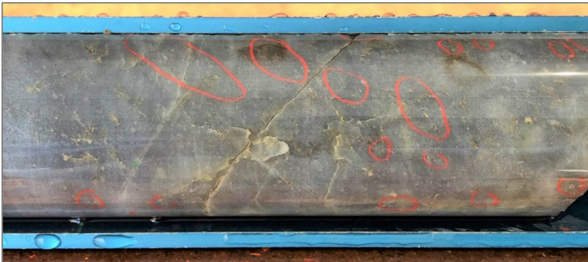
Photo 1: Typical silica-albite-sulphide Tura Lode mineralisation in BBRD1135 at 246.70m (assaying 184.64g/t Au); Multiple clusters of fine visible gold are circled in red; Core diameter is 47.60mm
