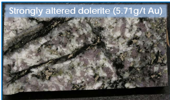
Quartz-biotite-albite-sulphide altered quartz dolerite (cf. Junction gold deposit, St Ives)
