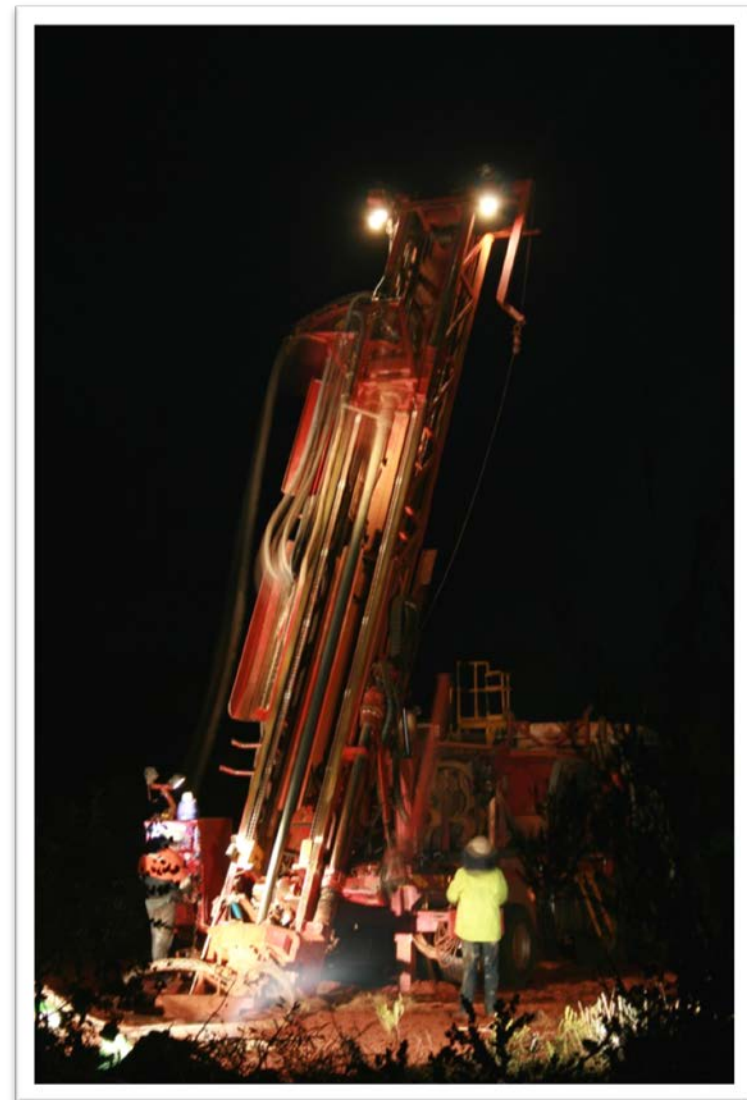
RC Drilling at Dexter Gold Project
